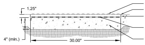
TekWay® ADA Dome-Tile 1/8" Radius at all sides of tile 1.25" recess for tile and Thinset mortar
